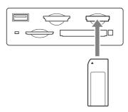
With the label facing up, fully insert the "Memory Stick" in the direction indicated by  $\blacktriangle$ .
